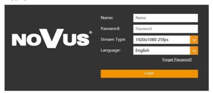
In this window, in order to login to camera, enter the user name root and the newly set administrator password. In the Stream type field user can select the stream that is displayed in the live view window after login. The Language field allows to change the interface language. The Forget Password option allows to log in to the camera if you forget the administrator password and for this is required to know the answers to the security questions (set in the next step).
