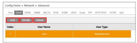
In order to delete the Onvif account, select the user by clicking on the appropriate row in the table, then click Delete button. Please note that deleting Onvif account means that the camera cannot be added to NMS software. Add button is used to create new Onvif account.
